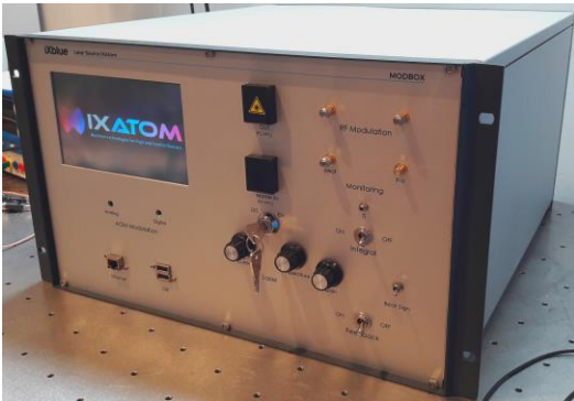
Figure 2: View of the CS-DSSB laser source developed by iXBlue
