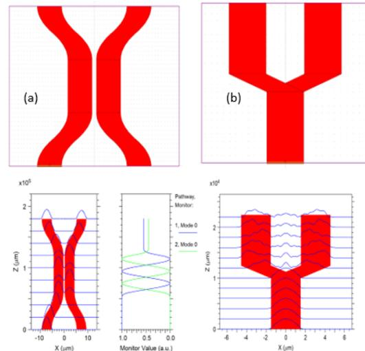
Figure 1: BPM simulation and results for the (a) Directional coupler and (b) Y branch splitter
