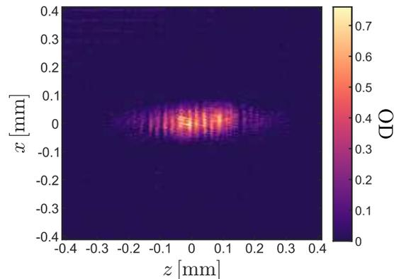
Figure 1: Interference fringes from two separate BECs expanding into each other in our apparatus. The BECs are formed in a double-well, then allowed to evolve in a cigar shaped trap.
