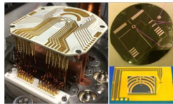
Figure 1: Current PCB (left), rf chip (top right) and atom-chip (bottom right).
